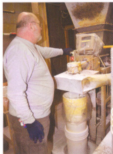
The operator fills and check weighs a 19 litre pail that will hold 23kg of finished product. The hopper in background holds 1135kg of product discharged from the ribbon blender on the floor above.
