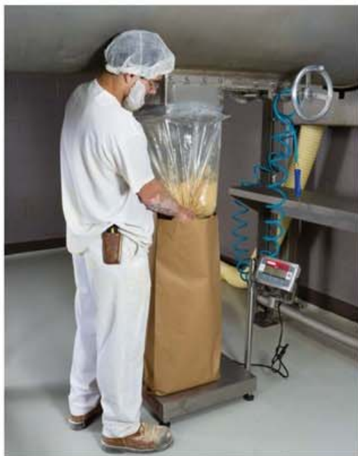
Blended product discharges into customer's final package.
