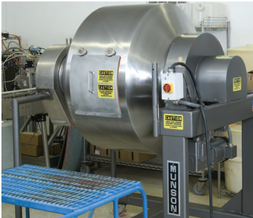
A 2-horsepower motor equipped with a high-efficiency helical gear reducer connected to a single-strand roller chain-and-sprocket drive powers the 10-cubic-foot-capacity rotary batch mixer.
