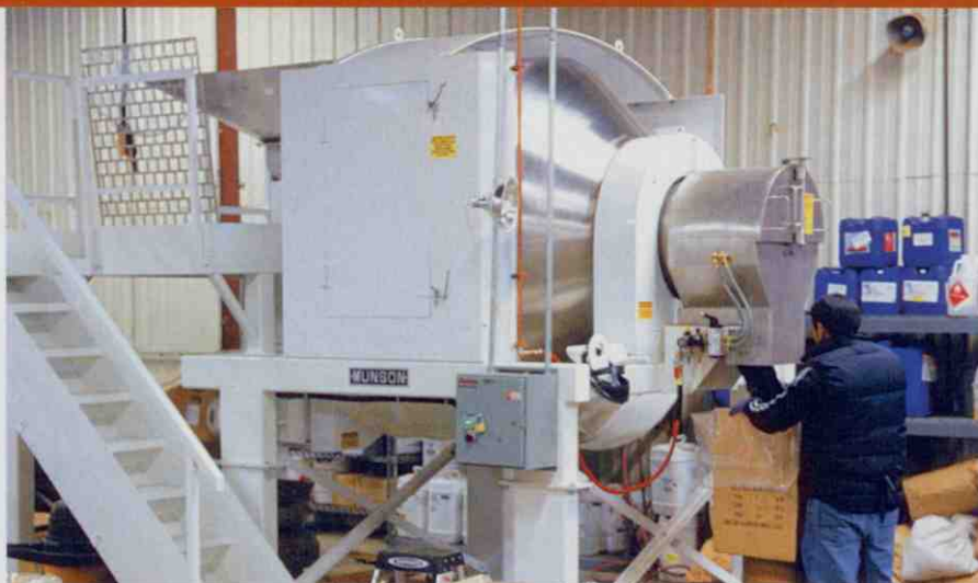
Top: This rotary blender is the heart of Harney's tea-blending facility.
