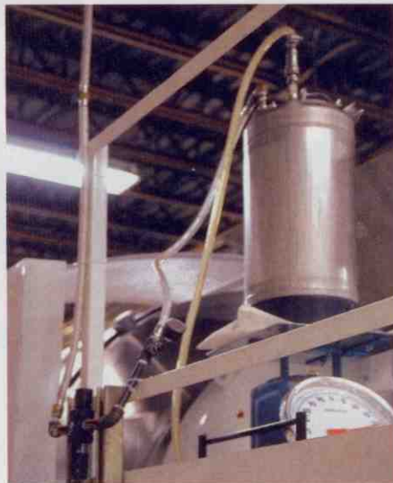
Liquid flavors are added from this vessel, located above the blender.
