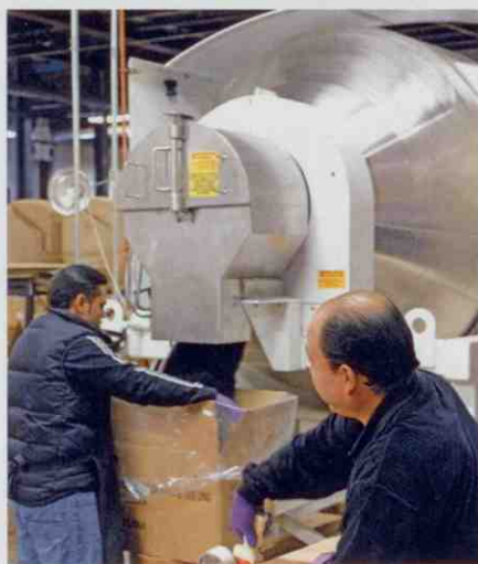
Top: This rotary blender is the heart of Harney's tea-blending facility.
