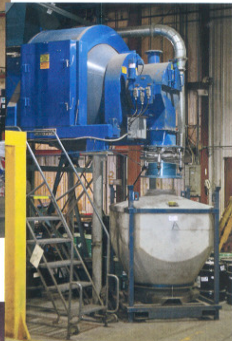
Blended powders are discharged from Rotary Batch Mixer into intermediate bulk containers before they are verified, then compacted to form "green" parts, ready for sintering. Broken pieces are loaded into a Pin Mill, also from Munson, reducing them into powders that are screened and blended with virgin
