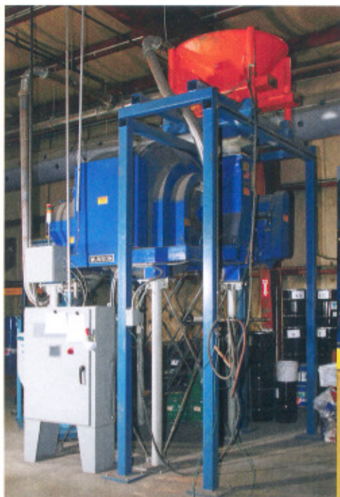
Munson Rotary Batch Mixer processes 5500 lb (2500 kg) batches of powdered metal components. Raw powder ingredients enter from surge hopper above and blended powders discharge into intermediate bulk
