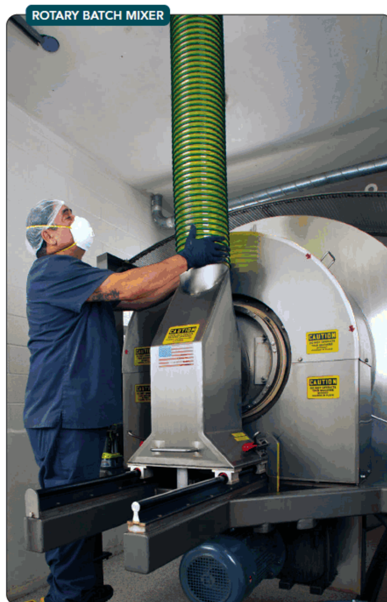
Figure 1. Unit blends ingredients in batches that range from 100 lb to 1,147 lb.
