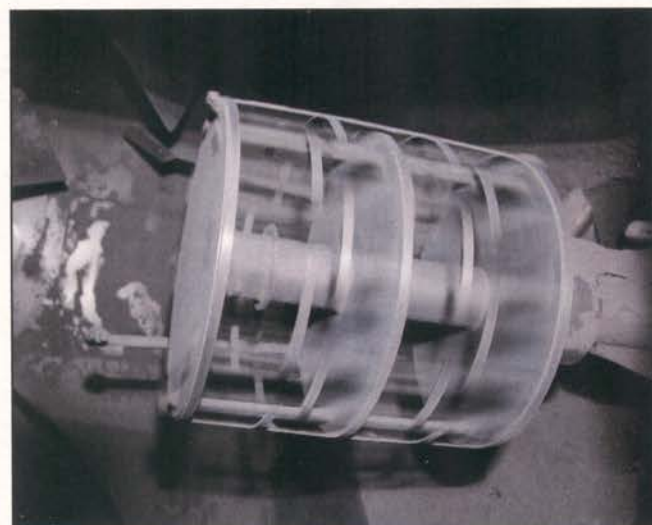
The cage-style intensifier at the inlet end of the mixer creates a high energy zone, ensuring homogenous blends.
