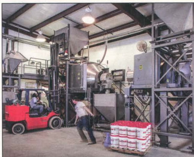
The two Munson rotary batch mixers are placed head to head.
