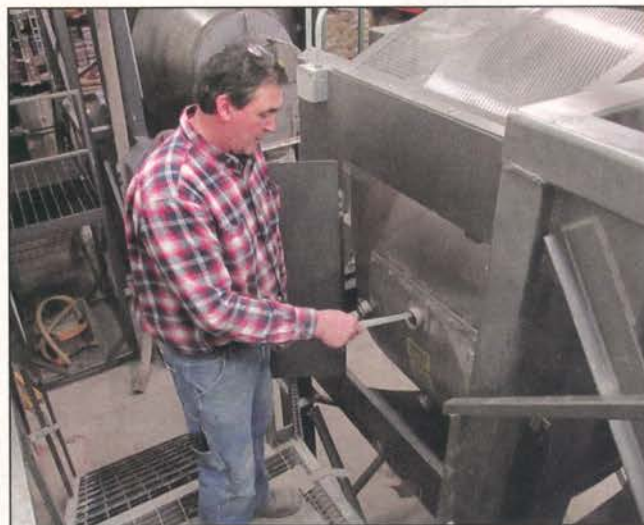
Jim Sacco takes batch samples from an inspection port for quality assurance checks.
