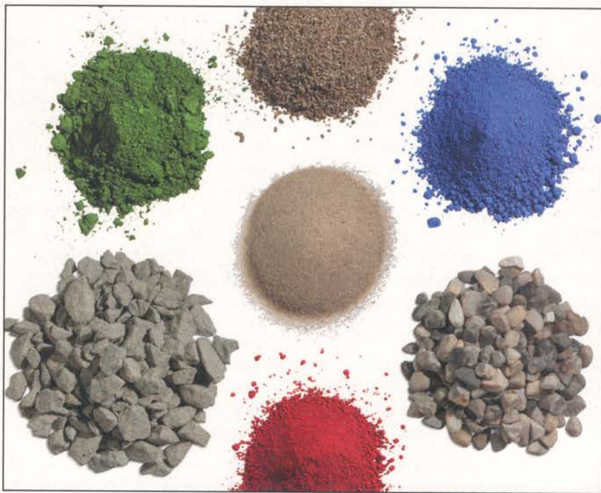
Raw materials and pigments for decorative concrete (clockwise from top): fine vermiculite, cobalt blue pigment, \frac{3}{16} - \frac{5}{16} -in. (4.7-7.9 mm) stone, red iron oxide pigment, \frac{3}{8} -in. (9.5 mm) local crushed stone, chromium oxide green pigment. Center, 70 mesh (0.21 mm) quartz.
