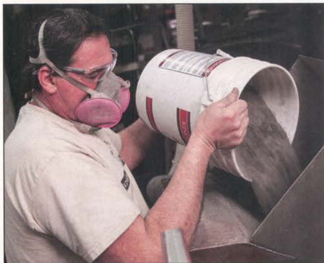
An operator introduces hand additives to the mixer.
