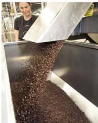
Continuous rotation of the drum during discharge prevents stratification of the batch. Photo courtesy Kicking Horse Coffee
