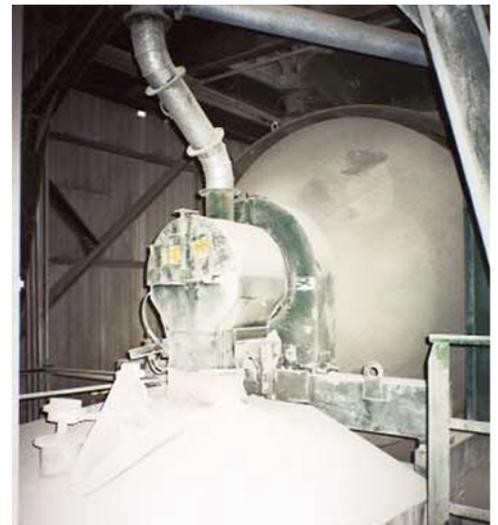
*The blender discharges the batch from the opposite side. Cycle times are typically 2 to 3 minutes. Working volume is 2.5 cubic meters and cleaning is easy.*
