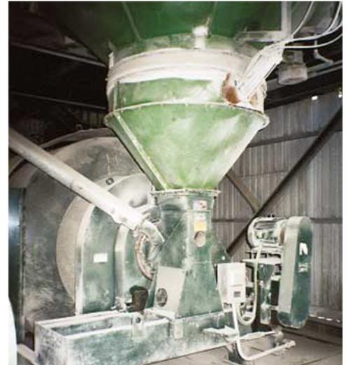
*After weigh-batching, the ingredients for the mortar enter the blender from above. The blender rotates during filling, blending, and unloading to prevent segregation.*
