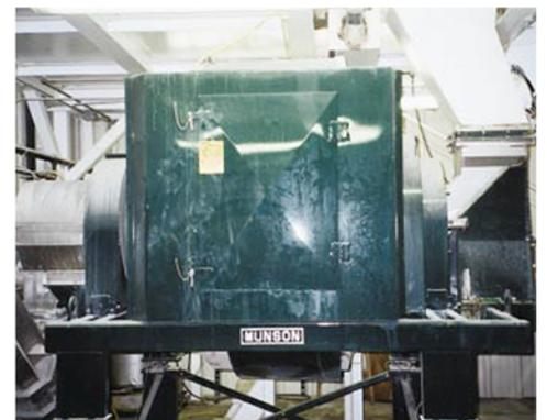
*This profile view of the blender shows the discharge chute (left), one of two drum access doors (center), and inlet chute (right).*
