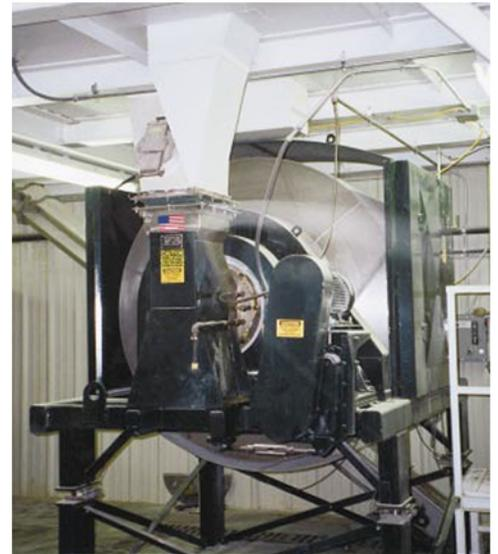
*Mounting the blender on load cells improves Akey's product formulation testing accuracy.*
